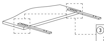
Secure each support stand by using 2x JCBB Bolt [1] and 2x M8 Flat Washer [2].
