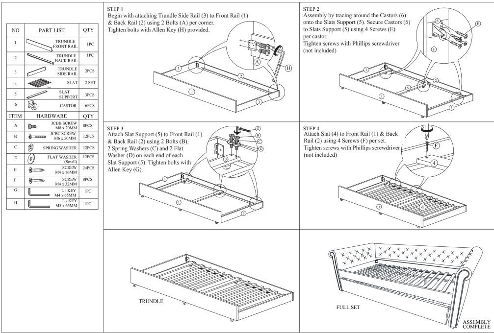
Please do not tighten the hardware until the entire assembly is completed.
