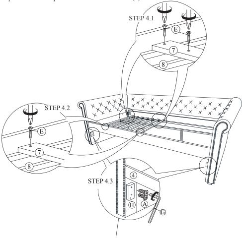
Step 4.3 attach the Stopper (H) to the front side of Side Panel (2) & (3) each side by securing with 2 Allen Bolt (A) using L-key (G) to avoid trundle pull out.
