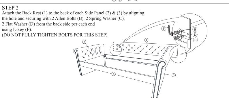
Please do not tighten the hardware until the entire assembly is completed.
