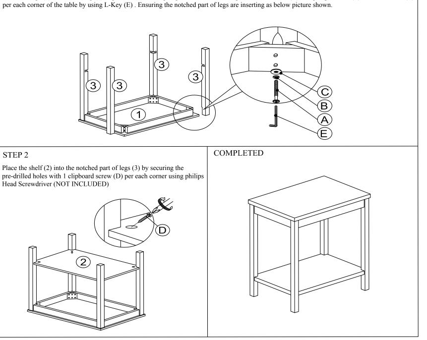
Insert the legs (3) to the table top (1) as picture shown. Aligning the hole and securing with 2 Allen Bolt (A), 2 Spring Washer (B), 2 Flat Washer (C)
