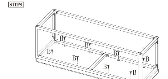
Note:Pls do not tighten all bolts until the products is assembled completely .
