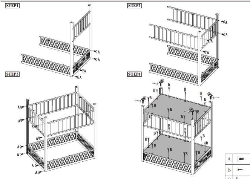
Note:Pls do not tighten all bolts until the products is assembled completely.
