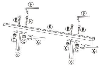
STEP 3 FIXING SIDE RAILS AND CENTRE SUPPORT BAR TO HEADBOARD AND FOOTBOARD
