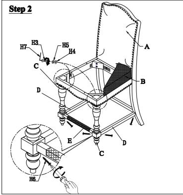
Step 1: Place the Chair Back (A) on the floor. Attach Seat Step 2: Attach the front legs to seat Cushion using flat washer (4), lock washer (5) and Allen Bolt (3) by using Allen Key (7). Attach the front, left side, right side of Stretcher to Right, left of Front Leg and Chair back by securing the Pan Head Screw (6) with Phillips screw drivers ( not included).
