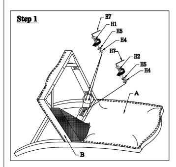
Cushion (B) to the Chair Back (A) by using Flat Washer (4), Lock Washer (5), Allen Bolt (1) into the holes at the corner block of the Seat Cushion (B). Insert Flat Washer (4), Lock Washer (5), Allen Bolt (2) into the rear bar of the seat frame. Secure by Allen Key (7).
