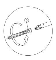
\*Assemble (B),(C),(G)&(H) panels, secure with Screw as shown.
