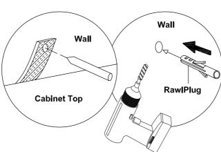
Drill a hole in the wall and insert the rawlplug.
