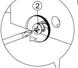
\*Attach Minifix Cap to both drawer side panels as shown.
