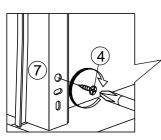
\*Assemble drawer slide, secure with screw as shown.
