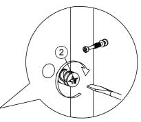
Assemble panels (I) in between panels (E) and (F), and secure them with Minifix (2) as shown.
