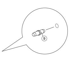
Attach 8pcs Shelf Support (9) to panels (A), (B), (J) & (K) as shown. Then place the adjustable panels (N) into cabinet as shown.
