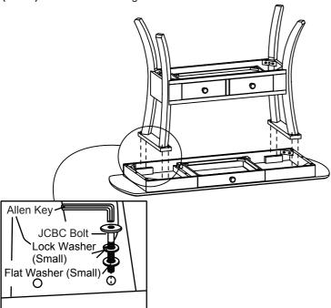
Turn the server upright. Check its balance and tighten all hex nut and bolts to complete the assembly.
