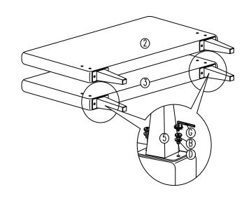
Attach the front rail (4) and back panel (1) to the right arm (2) and left arm (3). Aligning the holes and securing with 2 Allen Bolts (A) per each end by using L-key (H).
