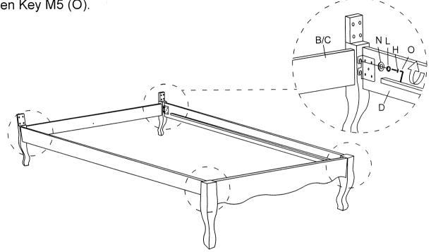
Insert JCBC M6 X 15mm (K) to L/Bracket (R) to Center Support (E) connection Headboard Leg Panel (B)/Footboard Panel (C) by Allen Key M4 (P).
