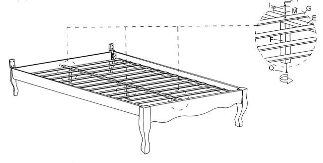
Insert CSK M4 X 32mm (S) to Bed slat (G) connection Side Rail Cleat (D).
