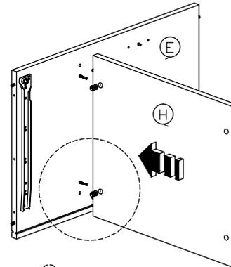
*\*Assemble panels, secure with Minifix as shown.*
