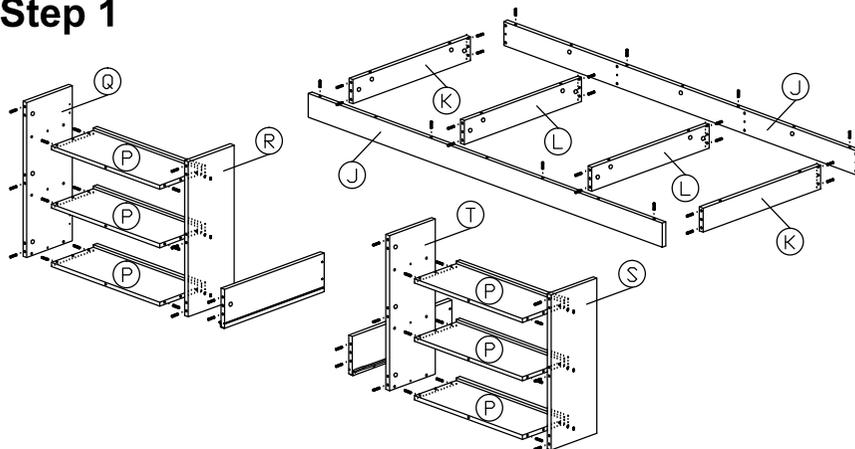
\*Install 100pcs Wood Dowel into all panels as shown.
