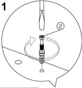
*\*Install minifix bolt to drawer front as shown.*
