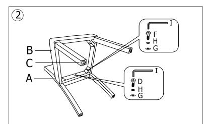
put the screws in the holes, tighten the screws, but not too tight, 90% is ok
