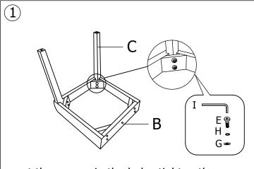
put the screws in the holes, tighten the screws, but not too tight, 90% is ok
