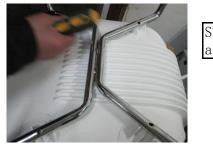
STEP1: Place the frame to the seat aiming to four screw holes.
