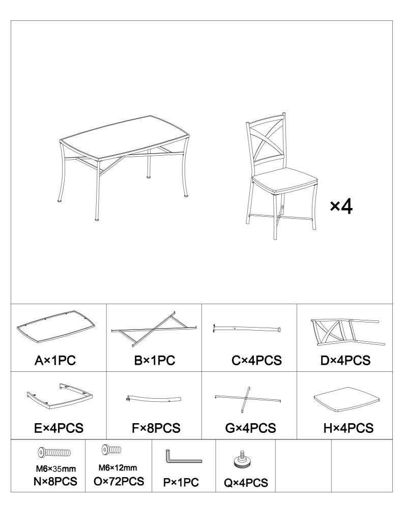
STEP 1 - USE SCREWS (Part O) to connect table feet (Part C), cross-bar (Part B) and table top (Part A) And then assemble adjustable feet (Part Q) to the table feet.
