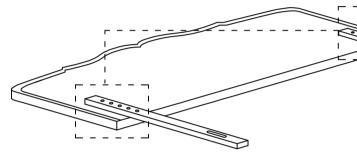
Secure each support stand by using 2x JCBB Bolt [1] and 2x M8 Flat Washer [2].
