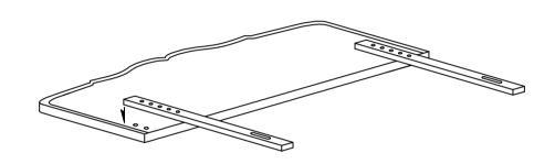
Align pre-drilled support stand holes over the pre-drilled headboard holes according to your desired headboard height
