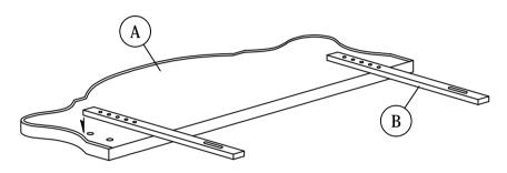
Align pre-drilled support stand holes over the pre-drilled headboard holes according to your desired headboard height
