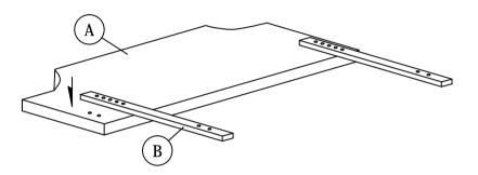
Align pre-drilled support stand holes over the pre-drilled headboard holes according to your desired headboard height
