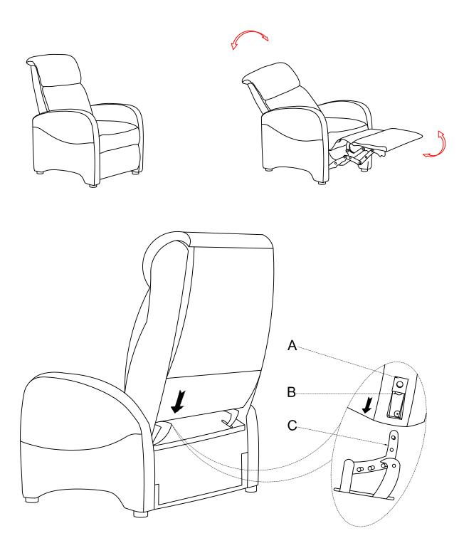
Align metal-clamp(A) on both sides of bottom of backrest to metal clamp(C) on base of seat cushion and push down so that metal lever(B) clicks in and backrest locks into place.
